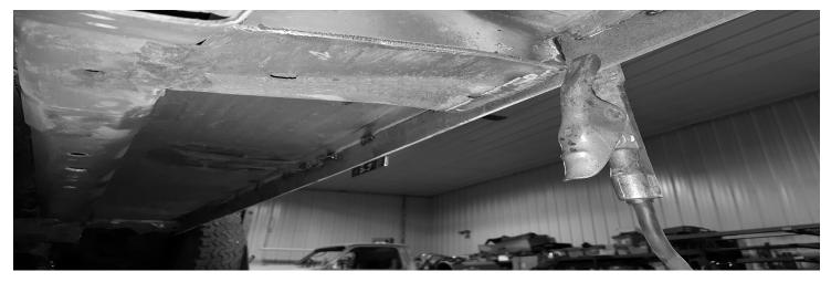
8) Once you've ensured a good fit from the inner ROCKer to the outer ROCKer, go ahead and weld the inner rocker. Stitch or skip welding is all that's really needed. A good seam sealer will seal up any areas not welded. You will want to weld the inside and outside of the inner ROCKer panels to the existing metal. Also be sure to weld the Torque boxes to the new inner ROCKer
