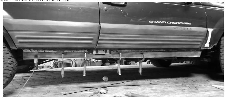
7) Position the inner ROCKer flat bar onto the jeep inner rocker. How high you set it will vary slightly, using the line you shown in step 5 is a very close guide. The best thing to do is tack weld or clamp it in place, then fit the outer ROCKer panel onto it to verify how they meet up as well as how straight it looks.
